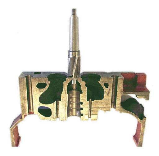
NOTE: Unless cracks extend to the valve seat area, valve seats do not need to be removed during nose plug machining and installation.
