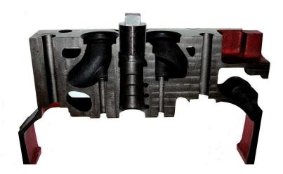
b) Turn the casting over, and coming in from the spring side of the casting, using the taper length drill (416-6156-26) and drill bushing (416-6156-19) drill the plug all the way through.
