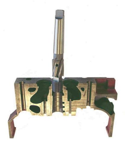
b) Now peen the outer rim of the plug, always peening away from the center of the plug. After peening the outer rim of the plug, smooth off the end of the plug. If the head is to be resurfaced later, bring the end of the plug down to about 1/32" above the face of the head. If there is not to be any later resurfacing of the head, then finish off the end other plug smooth with the face of the casting.
