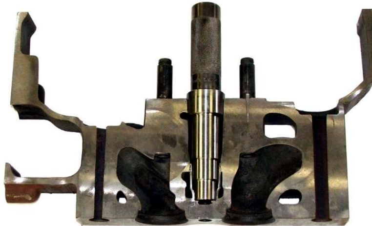
Sleeve Drive-In Tool inserting new Sleeve
